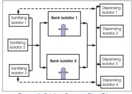
Figure 1: Existing Process Flow Diagram
