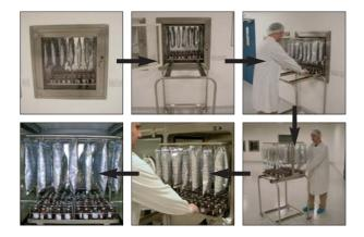
**5.** Each chamber has its own control panel mounted on the chamber front and on the push of a button, the door is pneumatically sealed and the cycle is initiated.
