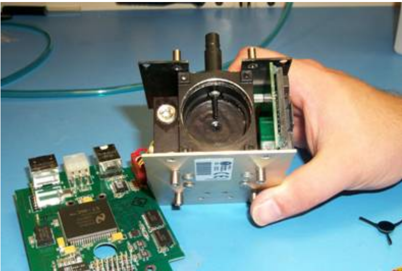
Figure 2. Teflon - coated, Airnet-510 XR optics chamber and internal components.
