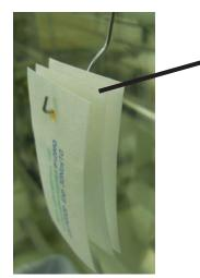
Plastic spacers have been placed on the wire hanger between each BI to ensure proper vapor flow around each BI unit.
