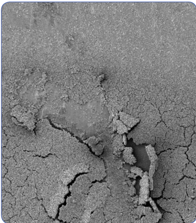
Image 4. Areas of dense and uneven microbial load (several layers thick) on a commercially available BI.
